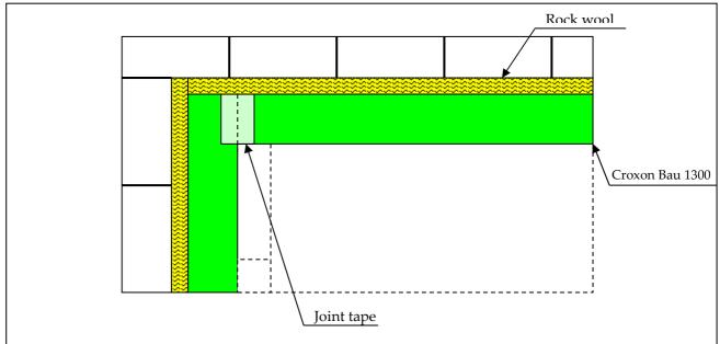
**Croxon Bau 1300** is a vibration elastic support base don recycled rubber for structural sound off in the building. Supplied cut into strips according to the plans in accordance with the load to bear, with the dynamic stiffness and resonant frequency required.
