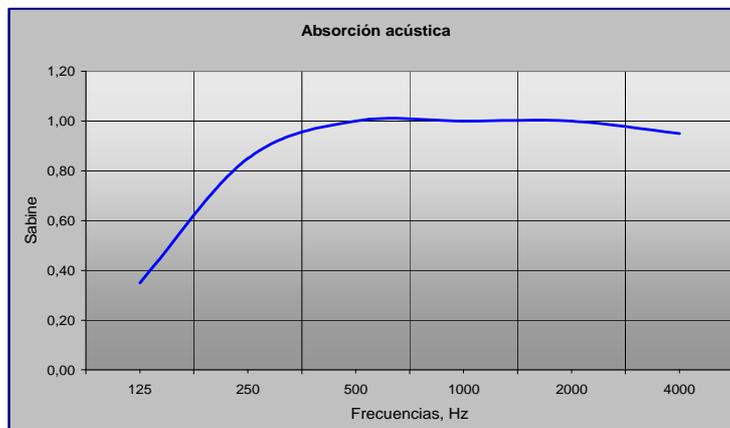
NCR ( $\alpha_w = 0,85$ ) Class C – ASTM C423
