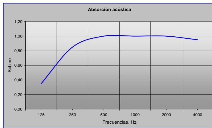
NCR ( $\alpha_w = 0,85$ ) Class C – ASTM C423
